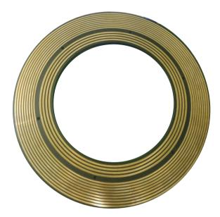
Pancake slip rings are designed for those have very limited height space but less limitation on diameter applications, also called platter separate slip rings or disc slip rings, they can utilize the existing bearings in the system to minimize the assembly height. In other words, a pancake slip ring can be without bearings.
